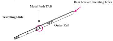
2 Mounting the rear 7" extension bracket as show in the picture below. Adjusting the extension bracket according to the mounting position you need in your cabinet. Align OB slots on the extension bracket with the (2) mounting holes at rear of Outer Rail. Secure the 7" extension to Outer Rail with (2) M4 Screw and Nuts. Do not tighten M4 screws yet.
